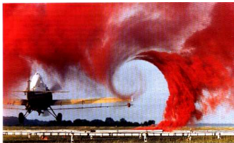
Aircraft trailing vortices
